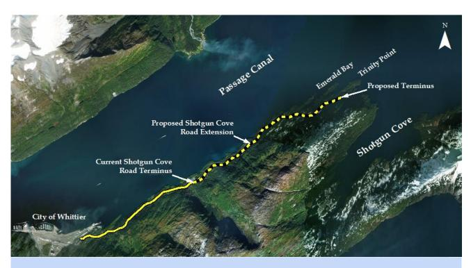
The proposed Shotgun Cove Road Extension will be constructed for approximately 2.5 miles, parallel to Passage Canal, from the existing Shotgun Cove Road terminus to Trinity Point. The proposed road will be two-lane and gravel.
