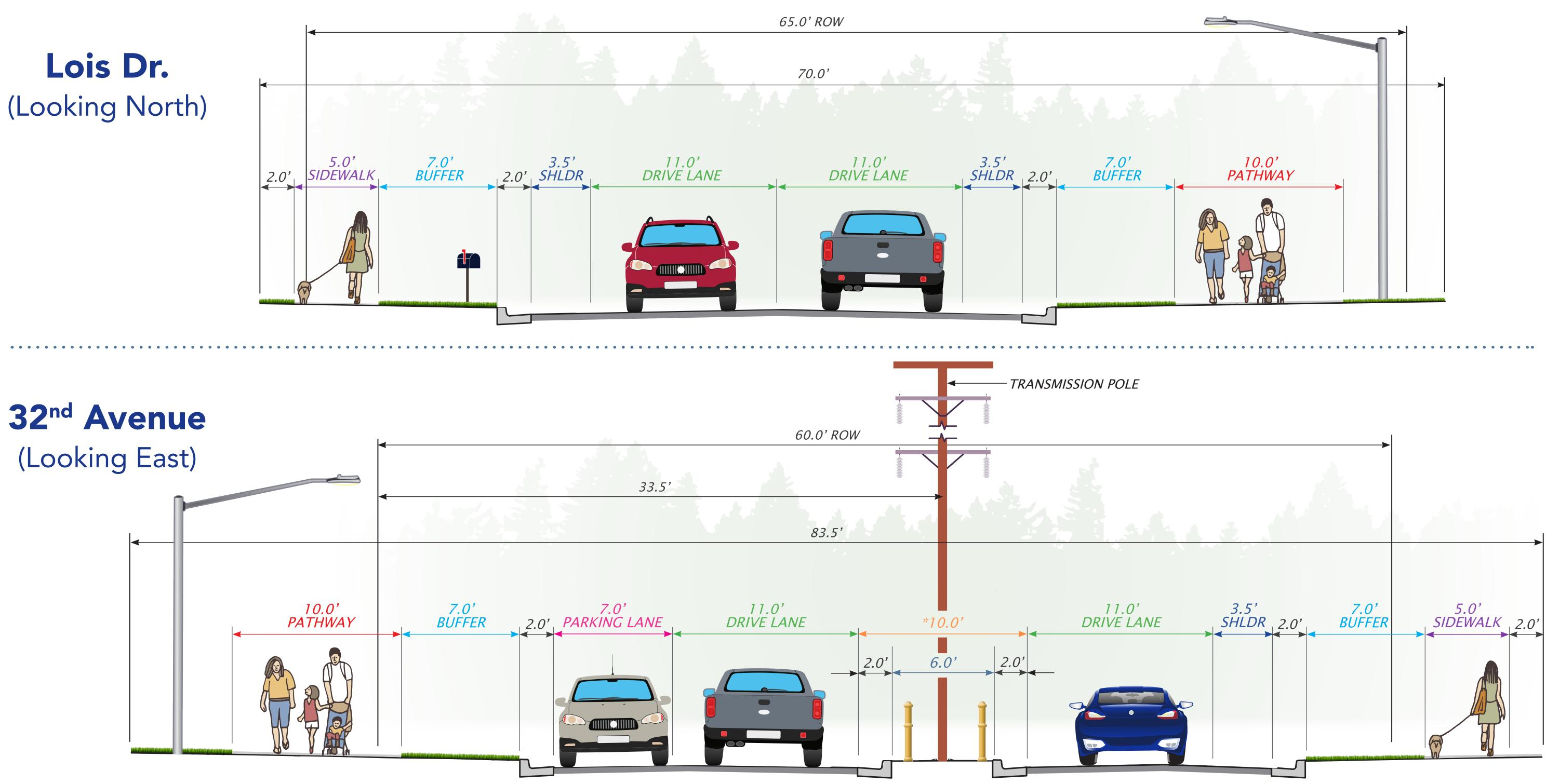
\*Center median only to be constructed at transmission and distribution poles
